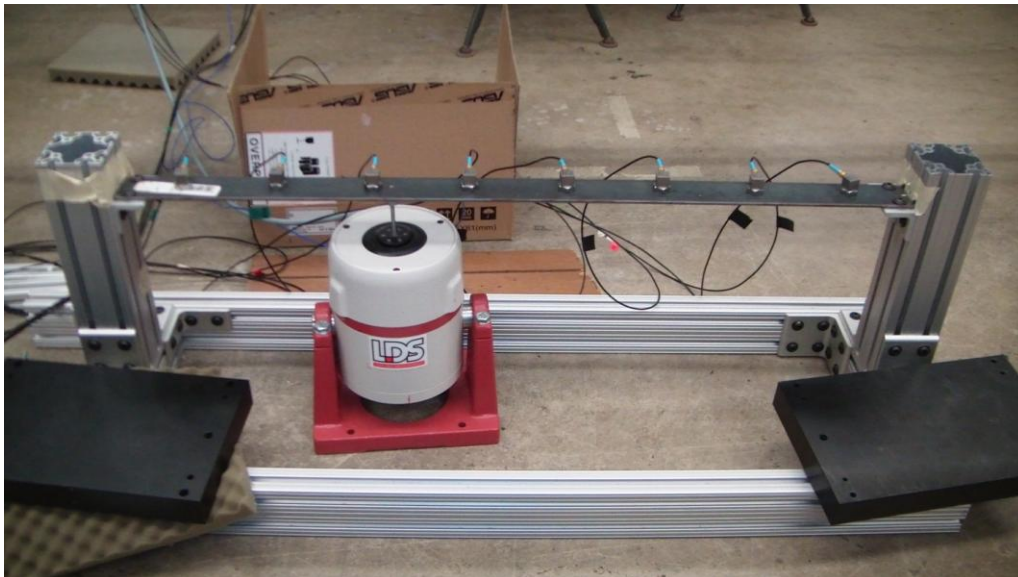
Figure 1 Test Setup for Laboratory Experimental Modal Testing
